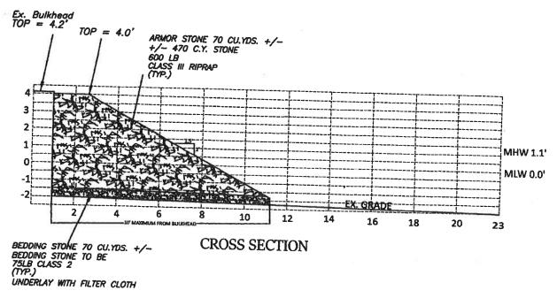
NOTE: RIPRAP SHALL NOT CONTAIN MORE THAN 10% BY WEIGHT OF THE SMALLEST SIZE STONE. FILTER CLOTH SHALL BE POLY FILTER-X OR AN EQUIVALENT WOVEN PLASTIC CLASS 'E'
