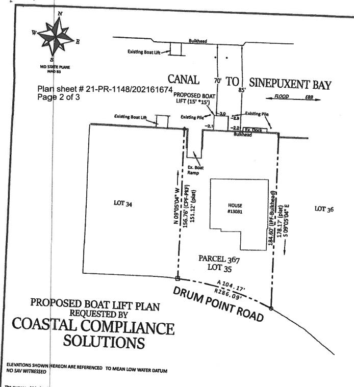
The purpose of this drawing is to obtain a permit for a boat lift only. This drawing is not a boundary survey and should not be relied upon for the establishment of property lines. This drawing does not guarantee title of CIVIL ENGINEERING & LAND SURVEYING
