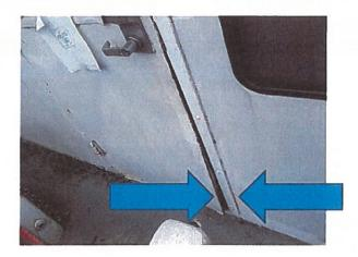
i) The latch on the port side tankage compartment escape hatch is broken.
