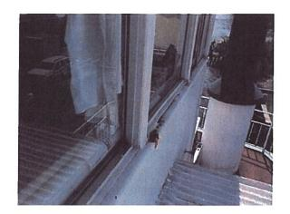
The fixed windows in the pilothouse are in good condition. However, the lower frame around the aft fixed windows is rusted.
