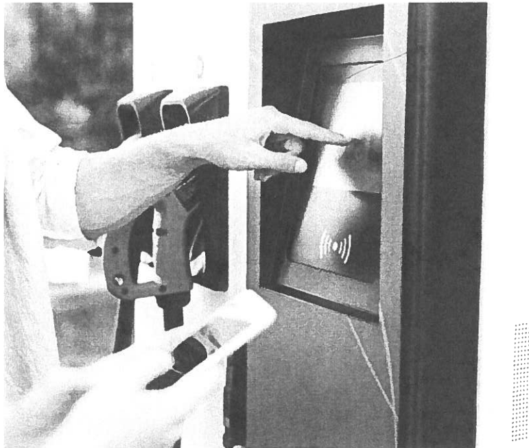
EV charger with Display Screen. Speech Output enabled is required under Section 508
