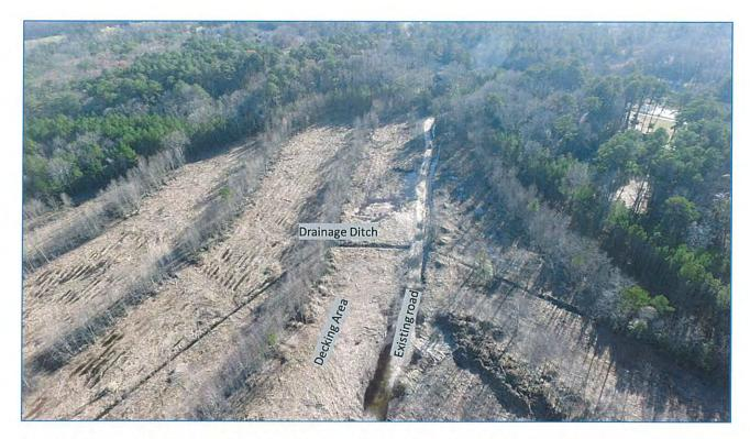
Figure 5. Photos of inoperative lateral drainage ditches, ditch running up to top of photo is operative and will not be affected by construction
